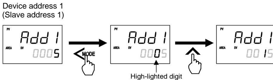
5. Press the SET key to store the new set value. The display goes to the next communication parameter. If the SET key is not pressed within 1 minute, the present display returns to the PV/SV monitor screen and the value set here returns to that before the setting is changed.
