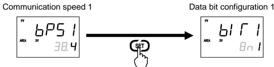
8. Set other communication parameters by the same procedure. After all the communications parameters are set, perform one of the following steps to make settings valid:
