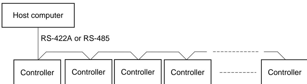
Maximum connections: RS-422A: Up to 31 controllers
