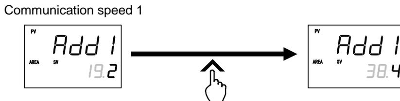
7. Press the SET key to store the new set value. The display goes to the next communication parameter. If the SET key is not pressed within 1 minute, the present display returns to the PV/SV monitor screen and the value set here returns to that before the setting is changed.
