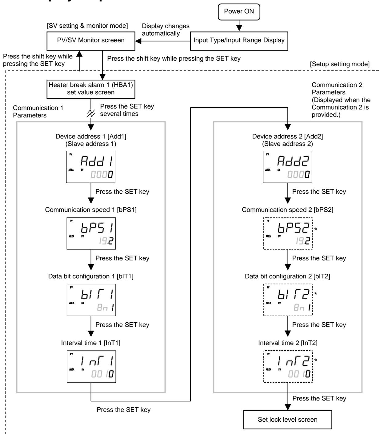
\* Displayed only when Communication 2 is used for Host communication. When Communication 2 is used for Host communication, refer to the ■ **Change the protocol of the Communication 2 port (P. 15)**.
