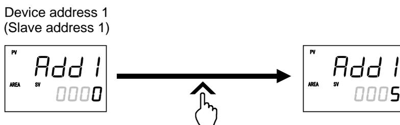
4. Press the shift key to high-light the tens digit, and press the UP key to change the digit to “1.”
