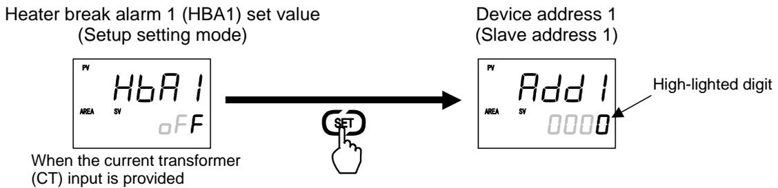
3. Set the Device address 1 (slave address 1). Press the UP key to change the number to 5.
