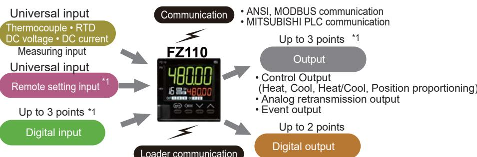
\*1 The number of inputs/outputs is limited depending on the specifications.
